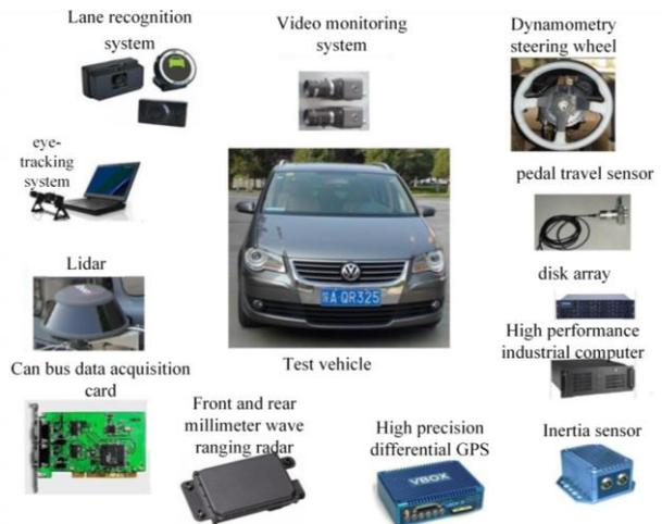
Figure 2. Multi-sensor platform vehicle
